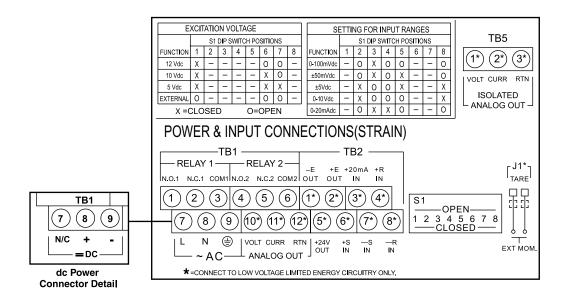
Figure 2-3. Connectors (AC-Powered and DC-Powered Detail)
