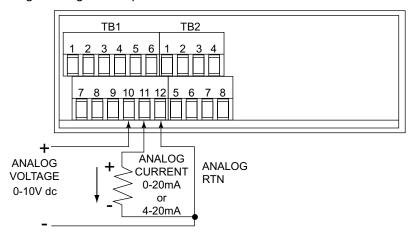
Figure 3-14. Analog Output Connections
