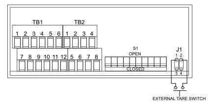
Figure 3-13. External Tare Connections
