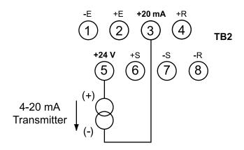
Figure 3-9. Current Input Connections with Internal Excitation
