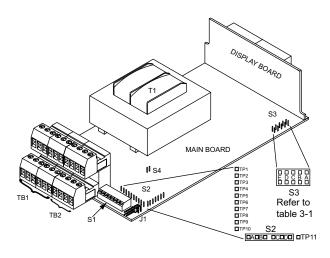
Figure 3-2. Main Board Jumper Positions
