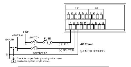
Figure 3-11. Main Power Connections - AC
