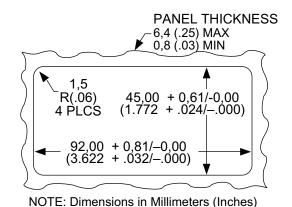
Figure 8-1 Meter Dimensions/ Panel Cutout
