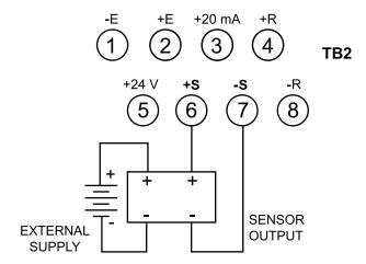
Figure 3-8. 4-Wire DC Input Connections with External Excitation
