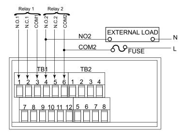
Figure 3-15. Relay Output Connections.
