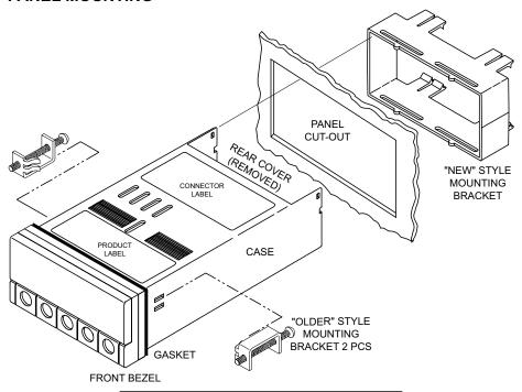
Figure 3-4. Meter - Exploded View
