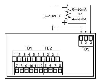
Figure 3-16. Isolated Analog Output Connections.
