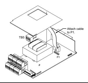
Figure 3-3. Upper Isolated Analog Output Option Board Installation
