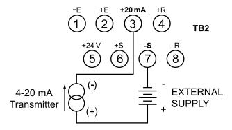
Figure 3-10. Current Input Connections with External Excitation
