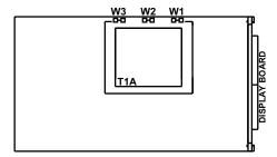
Figure 3.1 Main Board Power Jumpers
