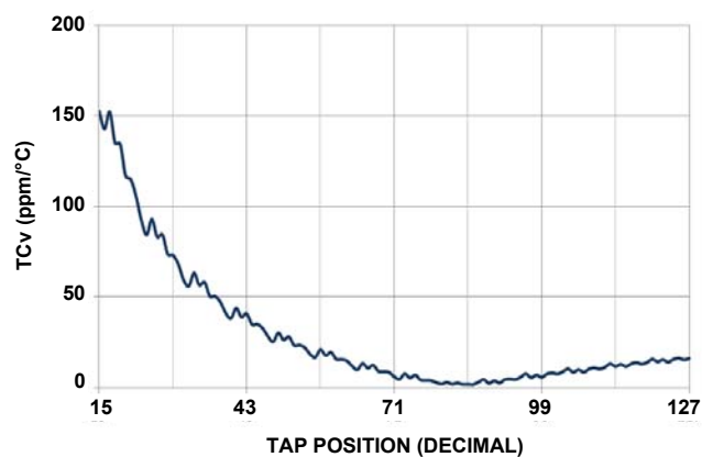
FIGURE 13. 10kΩ TCv vs TAP POSITION, V_{CC} = 3.3V
