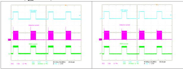
Figure 32. Dimming waveforms ( $F_{DIM} = 5 \text{ kHz}$ ) Figure 33. Dimming waveforms ( $F_{DIM} = 20 \text{ kHz}$ )
