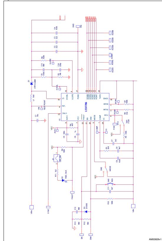
Figure 23. LED7706 demonstration board schematic
