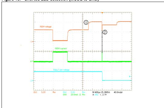
Figure 16. Shorted LED detection (MODE to GND)
