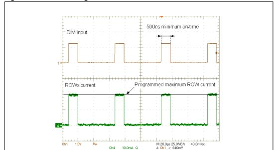
Figure 14. PWM dimming waveforms
