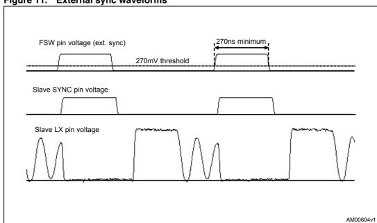
Figure 11. External sync waveforms
