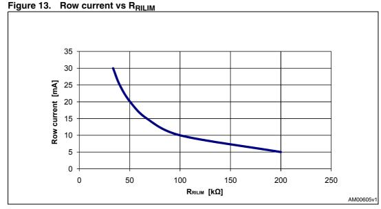
The maximum current mismatch between the rows is  $\pm 2 \%$  @  $I_{rowx} = 20 \text{ mA}$ .
