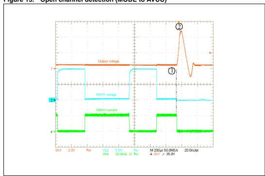
Figure 15. Open channel detection (MODE to AVCC)
