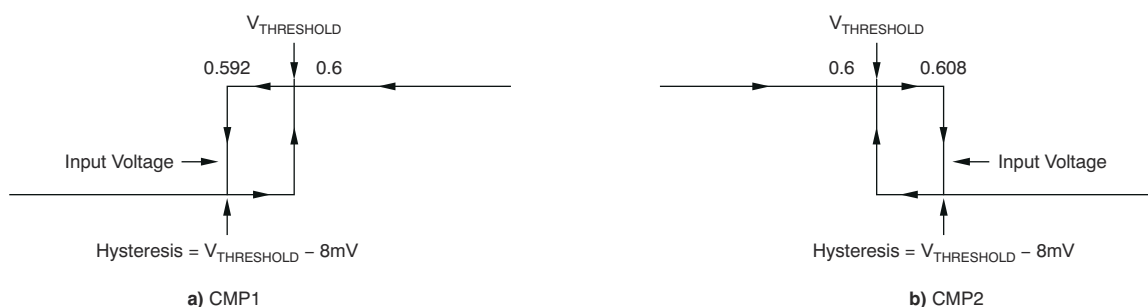
Figure 6-1. Comparator Hysteresis
