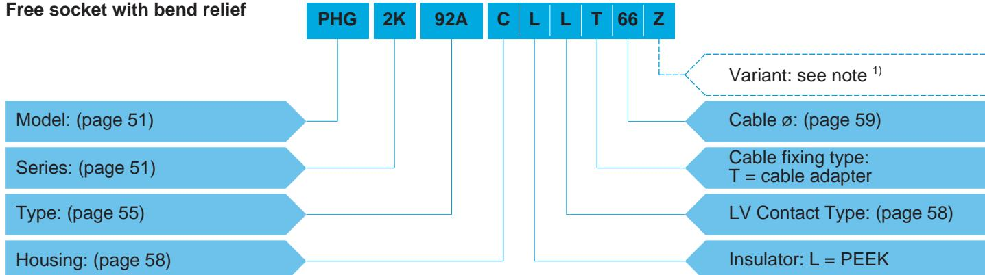
**PHG.2K.92A.CLLT66Z** = Free socket with key (G), 2K series, mixed type to accept 1 F2 type fibre optic contact and 2 low voltage contacts, chrome-plated brass housing, PEEK insulator, 2 female solder electrical contacts, cable fixing type T for 6.5 mm diameter cable, and nut for fitting a bend relief.
