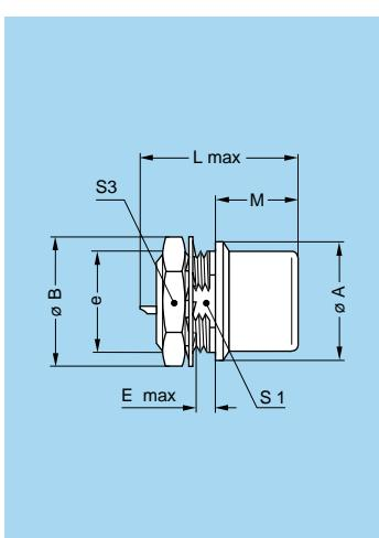
**Ehg Fixed socket, nut fixing, key (G) or keys (A...L and R), visible shell**
