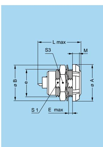
**Ecg Fixed socket, with two nuts, key (G) or keys (A...L and R), (back panel mounting)**
