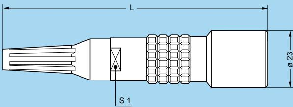
**PHW.3K** Free socket, keys (W), cable adapter, with bend relief
