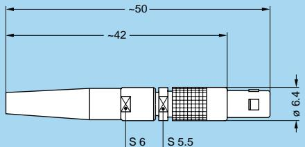
**PKG.00** Fixed socket, nut fixing, key (G) or key (B), with bend relief
