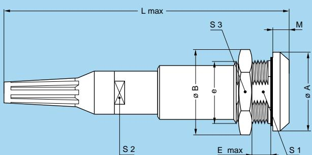
**PKG** Fixed socket, nut fixing, key (G) or keys (A...F, L and R) and cable adapter and nut for fitting a bend relief
