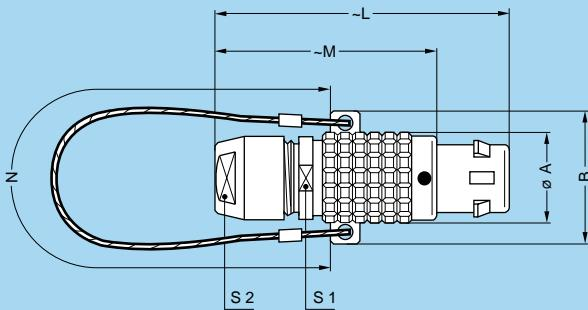
**FNG** Straight plug, key (G) or keys (A...L and R) and cable collet with lanyard release
