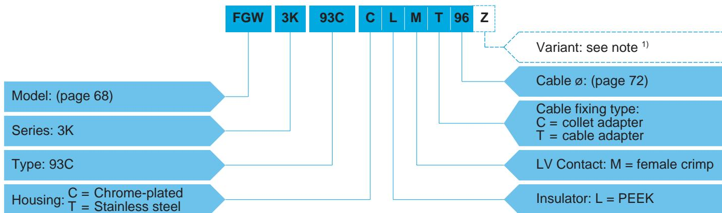
**FGW.3K.93C.CLMT96Z** = Straight plug with keys (W), 3K series, mixed type to accept 2 F2 type fibre optic contacts, 2 power and 2 signal electrical contacts, chrome-plated brass housing, PEEK insulator, female crimp signal contacts, cable fixing type T for 9.2 mm diameter cable, and nut for fitting a bend relief.
