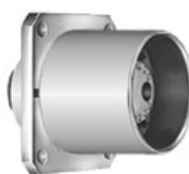
**EDG** Fixed socket with square flange, key (G) or keys (A...F, L and R), protruding shell and earthing tag, screw fixing
