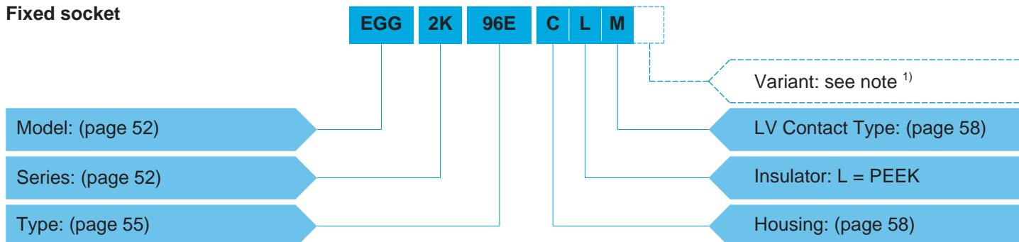
**EGG.2K.96E.CLM** = Fixed socket with key (G), 2K series, mixed type to accept 1 F1 type fibre optic contact and 6 low voltage contacts, chrome-plated brass housing, PEEK insulator, 6 female crimp electrical contacts.
