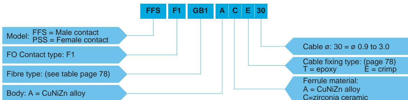
**FFS.F1.GB1.ACE30** = Male F1 type fibre optic contact, ferrule bore diameter of 235 µm, ferrule made of zirconia ceramic, crimp type cable fixing for a cable diameter of 0.9 mm to 3.0 mm.
