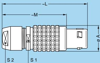
**FGG** Straight plug, key (G) or keys (A...L and R) and cable collet
