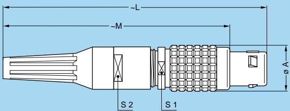
**FGG** Straight plug, key (G) or keys (A...L) cable collet and nut for fitting a bend relief
