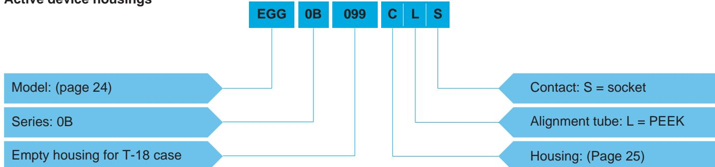
**EGG.0B.099.CLS** = Fixed active device housing, nut fixing, with key (G), 0B series, empty housing for TO-18 case, chrome-plated brass housing, PEEK alignment tube, socket contact.
