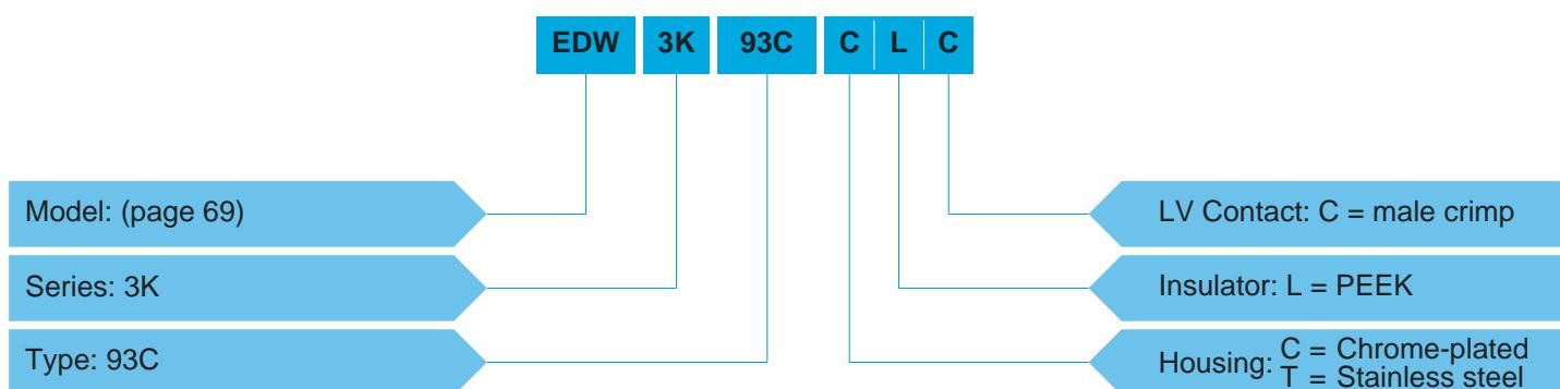
**EDW.3K.93C.CLC** = Fixed socket with rear square flange, keys (W), 3K series, mixed type to accept 2 F2 type fibre optic contacts, 2 power and 2 signal electrical contacts, chrome-plated brass housing, PEEK insulator, male crimp signal contacts.
