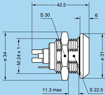
**ENW.3K** Fixed socket, nut fixing, keys (W), and earthing tag
