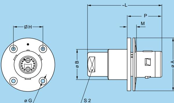
**FXG** Fixed plug with round flange, four holes fixing, key (G) or keys (A...F, L and R)
