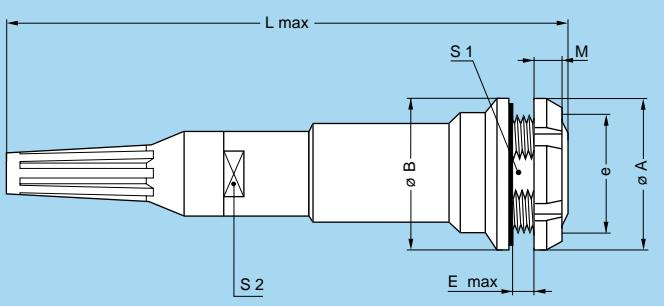
**PEG** Fixed socket, nut fixing, key (G) or keys (A...F, L and R), cable adapter and nut for fitting a bend relief (back panel mounting)
