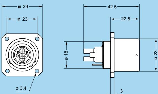
**EDW.3K** Fixed socket with rear square flange (4 holes fixing), keys (W), and earthing tag
