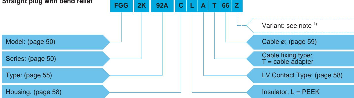
**FGG.2K.92A.CLAT66Z** = Straight plug with key (G), 2K series, mixed type to accept 1 F2 type fibre optic contact and 2 low voltage contacts, chrome-plated brass housing, PEEK insulator, 2 male solder electrical contacts, cable fixing type T for 6.5 mm diameter cable, and nut for fitting a bend relief.
