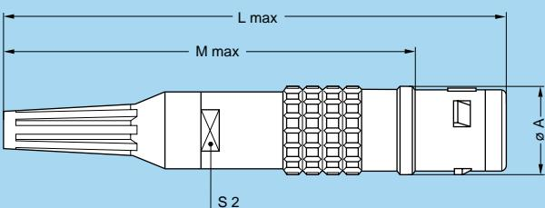
**FGG** Straight plug, key (G) or keys (A...F, L and R), cable adapter and nut for fitting a bend relief
