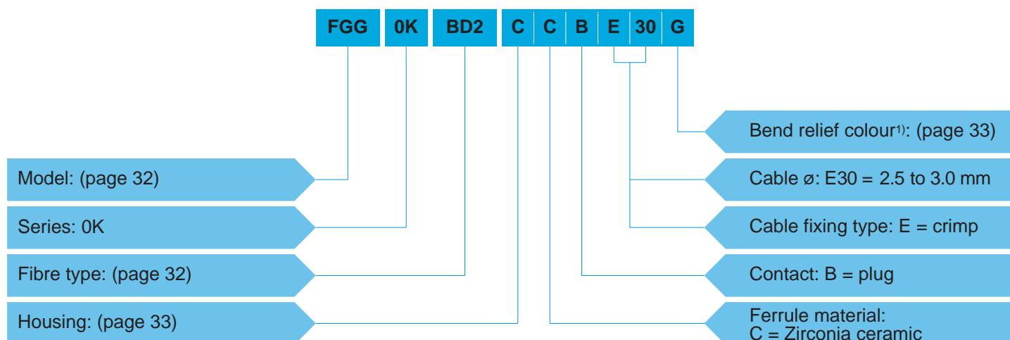
**FGG.0K.BD2.CCBE30G** = Straight plug with key (G), 0K series, F2 fibre optic contact, ferrule hole ø 128 µm, chrome-plated brass housing, zirconia ceramic ferrule, plug type contact, crimp type cable fixing for 2.5 to 3.0 mm diameter cable, and gray bend relief.
