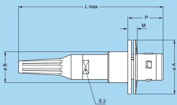
**FMG** Fixed plug with round flange, four hole fixing, key (G) or keys (A...F, L and R), cable adapter and nut for fitting a bend relief
