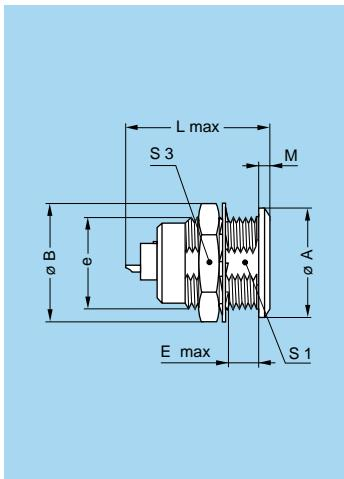
**Egg Fixed socket, nut fixing, key (G) or keys (A...L and R)**
