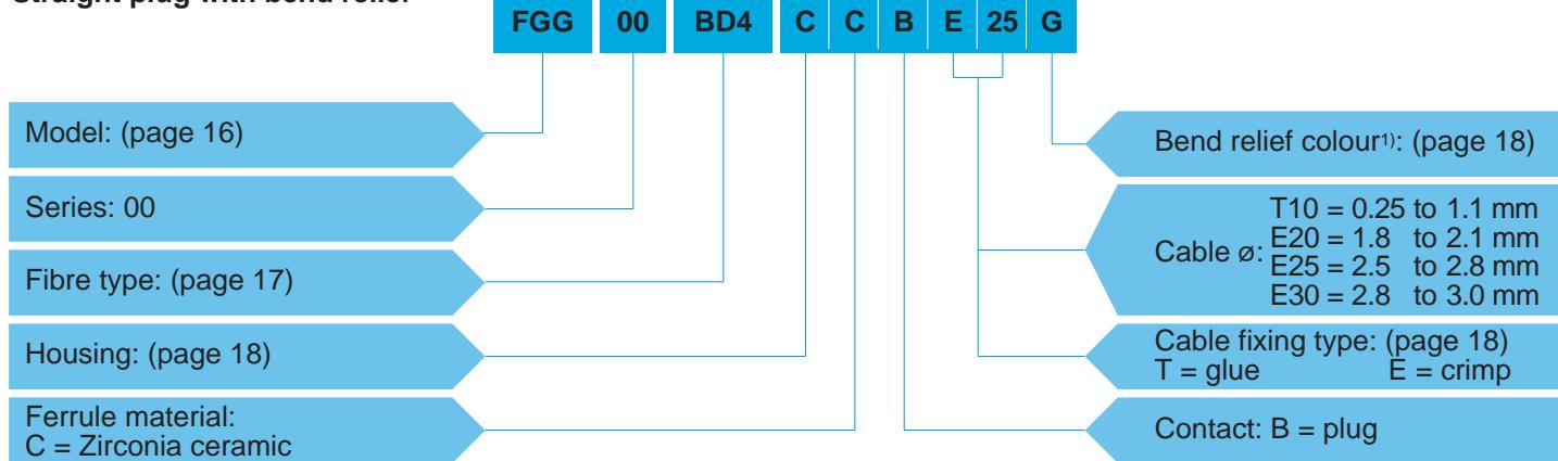
**FGG.00.BD4.CCBE25G** = Straight plug with key (G), 00 series for single-mode or multi-mode fibres, F4 fibre optic contact, ferrule hole diameter 128 µm, chrome-plated brass housing, zirconia ceramic ferrule, plug type contact, crimp type cable fixing for 2.5 to 2.8 mm diameter cable, and gray bend relief.
