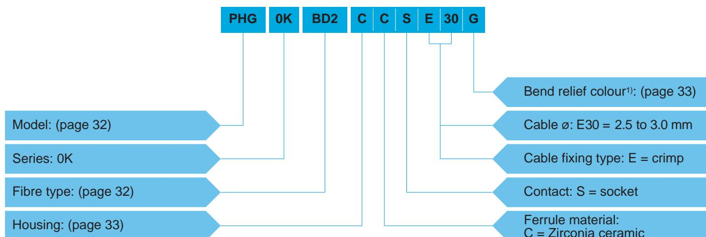
**PHG.0K.BD2.CCSE30G** = Free socket with key (G), 0K series, F2 fibre optic contact, ferrule hole ø 128 µm, chrome-plated brass housing, zirconia ceramic ferrule, socket type contact, crimp type cable fixing for 2.5 to 3.0 mm diameter cable, and gray bend relief.
