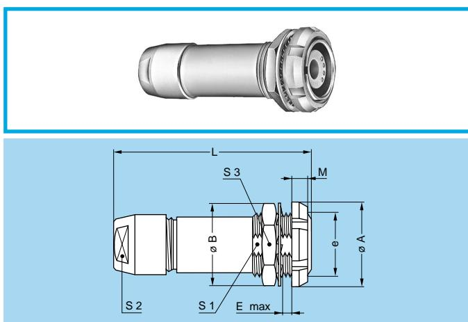
**PFG** Fixed socket, with two nuts, key (G) or keys (A...L and R) and cable collet, (back panel mounting)
