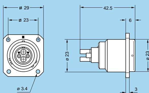
**EBW.3K** Fixed socket with front square flange (4 holes fixing), keys (W)
