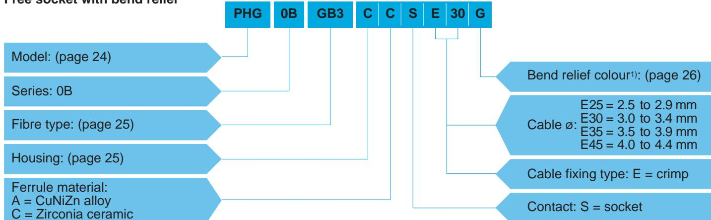
**PHG.0B.GB3.CCS30G** = Free socket with key (G), 0B series, F3 fibre optic contact, ferrule hole diameter 235 µm, chrome-plated brass housing, zirconia ceramic ferrule, socket type contact, crimp type cable fixing for 3.0 to 3.4 mm diameter cable, and gray bend relief.
