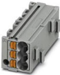
Marshalling patchboard, Nom. voltage: 500 V, Nominal current: 17.5 A, Cross section: 0.14 mm<sup>2</sup> - 2.5 mm<sup>2</sup>, AWG: 12 - 26, Connection type: Push-in connection, Number of positions: 1, Number of connections: 6, Width: 11 mm, Length: 12.2 mm, Color: gray, Color of connection elements: gray, Assembly: for snapping onto a DIN rail adapter, for snapping onto a cover flange
