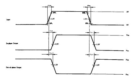
Notes) i. Input pulse:  $t_{TLH} \le 15$ ns,  $t_{THL} \le 6$ ns, PRR = 1MHz, duty cycle=50%.
