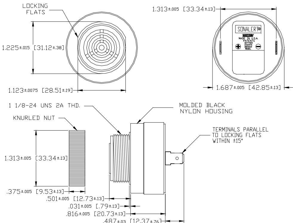
NOTE: MOUNTING- REMOVE BLACK PLASTIC NUT AND INSERT THREADED FRONT THROUGH 1.25" HOLE PUNCHED IN PANEL, IF ORIENTATION IS NEEDED, NOTE LOCKING FLATS ON DRAWING. SCREW NUT BACK ON. DO NOT OVERTIGHTEN.
