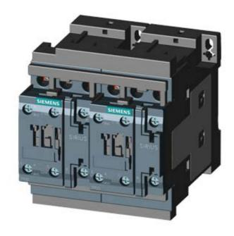
REV. COMB., AC3, 15KW/400V DC24V 3-POLE, SZ SO SCREW TERMINAL ELECTR. AND MECH. INTERLOCK 2NO INTEGR.
