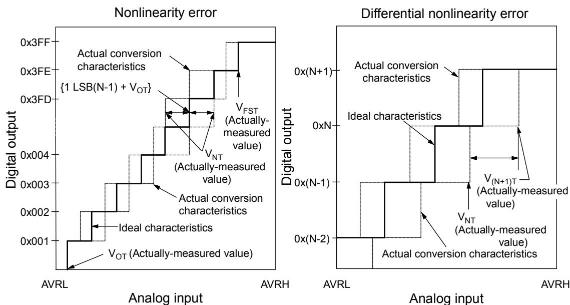
$$\text{Nonlinearity error of digital output } N = \frac{V_{NT} - \{1\text{LSB} \times (N - 1) + V_{OT}\}}{1\text{LSB}} \text{ [LSB]}$$
