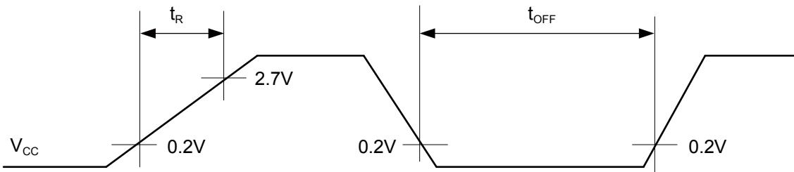
If the power supply is changed too rapidly, a power-on reset may occur. We recommend a smooth startup by restraining voltages when changing the power supply voltage during operation, as shown in the figure below.
