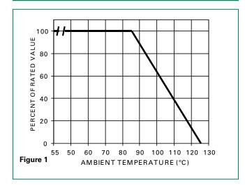
For applications exceeding 85°C ambient temperature, the peak surge current and energy ratings must be reduced as shown above.
