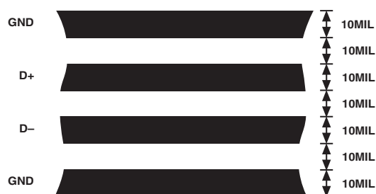
Figure 6. Arrangement of Signal Tracks
