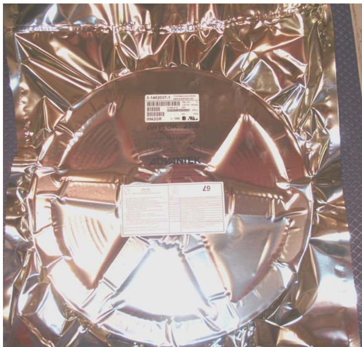
Fig. 2: Dry packed SMT relays
