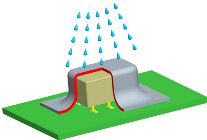
Fig. 11: Coating of relays on PCB's
