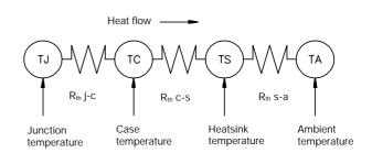
Thermal resistance: R<sub>th</sub> j-c = junction to case  $R_{th}$  c-s = case to heatsink  $R_{th}$  s-a = heatsink to ambient
