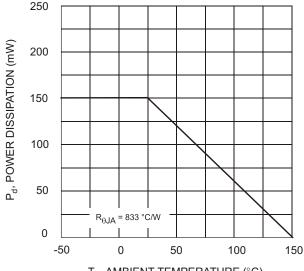
T<sub>A</sub>, AMBIENT TEMPERATURE (°C) Fig. 1, Derating Curve - Total
