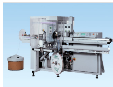
Ferrule Applicator (CA10) in Automatic Wire Processing Machine
