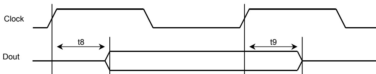
Figure 18-5. To/From High-Z Delay Definitions (Rising Clock Edge)
