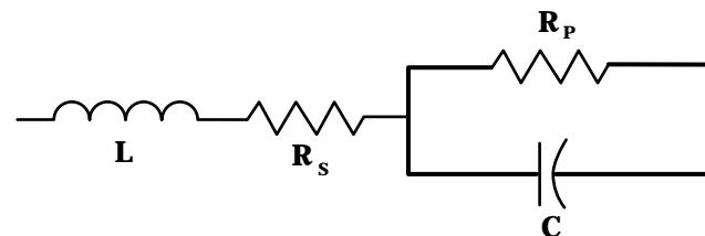
**Reactance** – Since the insulation resistance ( $R_p$ ) is normally very high, the total impedance of a capacitor is:
