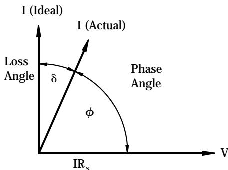
In practice the current leads the voltage by some other phase angle due to the series resistance  $R_s$ . The complement of this angle is called the loss angle and:
