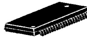
Outline 42P2R-A 0.8mm Pitch 450mil SSOP (8.4mm x 17.5mm x 2.0mm)
