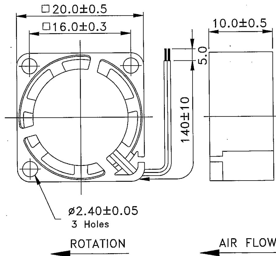
LEAD WIRES : UL 1571, AWG28 , L=140 +/- 10 MM
