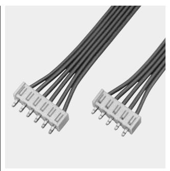
The SDN connector is a 3.96mm (.156") pitch board-in crimp style connector capable of connecting a wide variety of circuits including signal and power supply circuits. The connector features a slim, low-profile design. In addition, it has an exclusive lance construction to reduce insertion force, thus substantially improving the working efficiency in mounting the contact.
