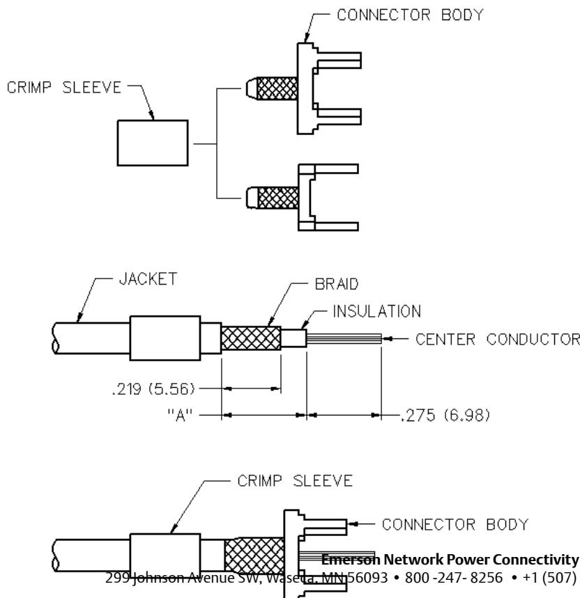
1. Identify connector parts. (2 piece parts)
