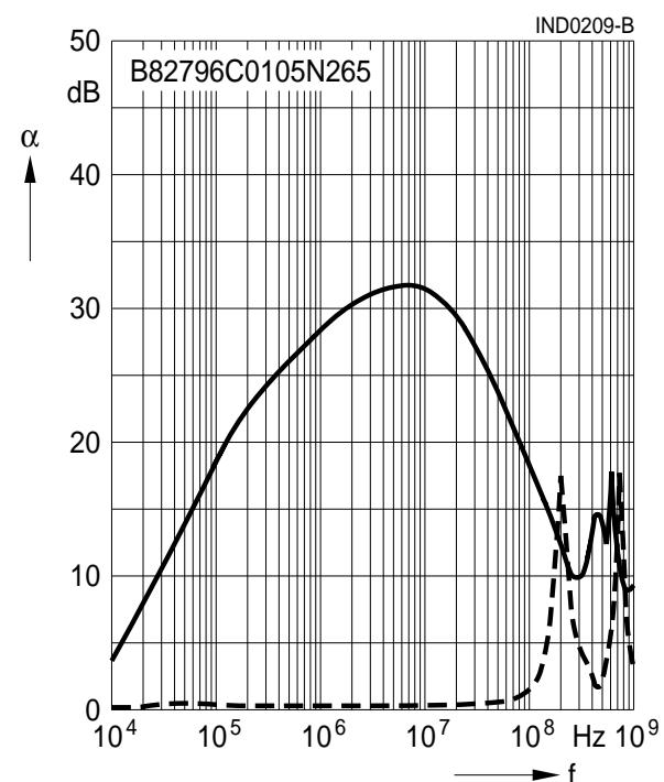
**Insertion loss  $\alpha$  (typical values at  $|Z| = 50 \Omega$ ,  $20^\circ\text{C}$ )**
