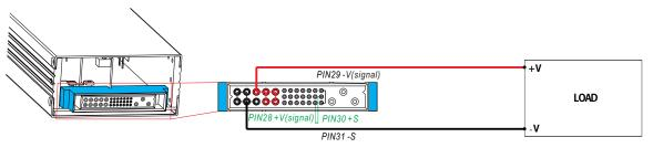
2. Output Voltage Programming (or, PV / remote voltage programming / remote adjust / margin programming / dynamic voltage trim)
