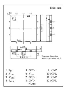
Note) 1. The reverse of the device is solderd to the plate
