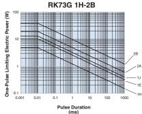
The maximum applicable voltage is equal to the max. overload voltage. Please ask us about the resistance characteristic of continuous applied pulse. The pulse endurance values are not assured values, so be sure to check the products on actual equipment when you use them.
