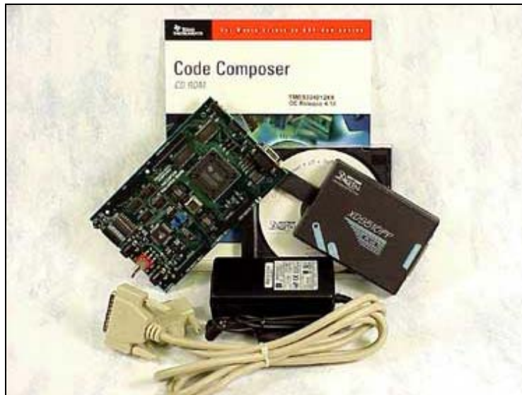
EVM320F240 + Power Supply + XDS510PP PLUS Emulator + Code Composer Studio for the C2xxx
