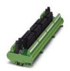
32-channel module with 1-conductor screw connection and a fuse in each signal path (5 x 20 mm). The voltage supply and the 50-pos. system connection are designed redundantly. Suitable for the Yokogawa ADV151 and ADV551 cards.
