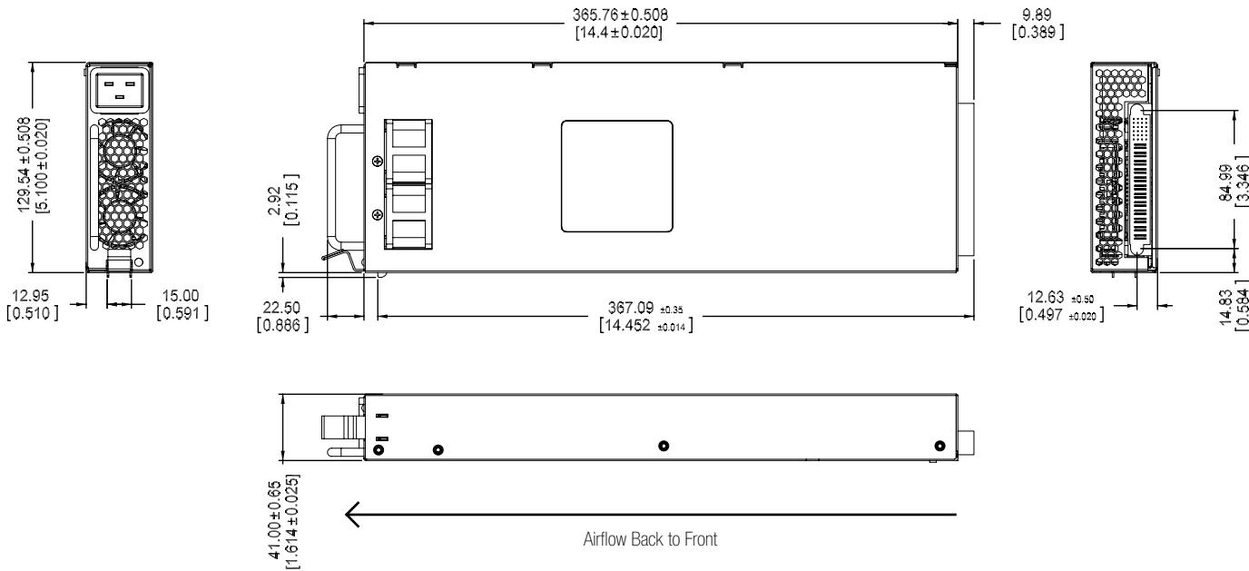
AC Input Connector: The AC input connector is standard IEC320 C20 (20A).
