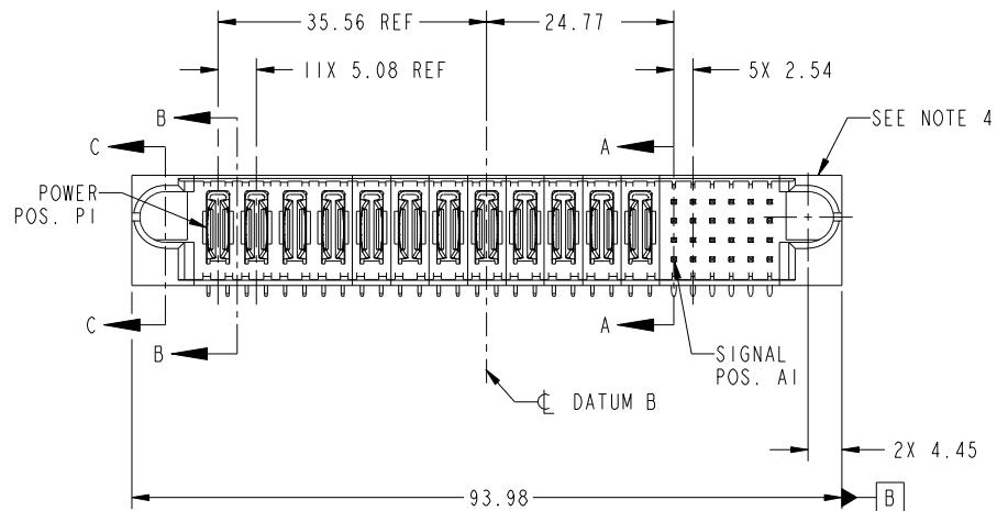
**DC OUTPUT VERTICAL CONNECTOR MATE ON BACKPLANE (backplane view)**
