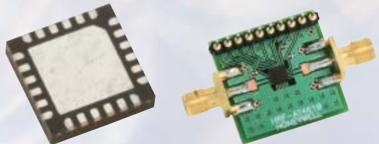
Package Photo and HRF-AT4610 Eval Board
