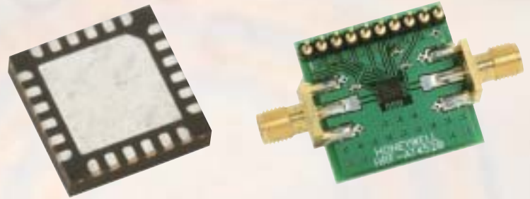
Package Photo and HRF-AT4520 Eval Board
