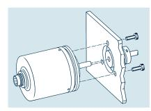
...by screw fastening directly onto the encoder flange
