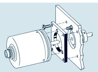
...by screw fastening onto a mounting adapter
