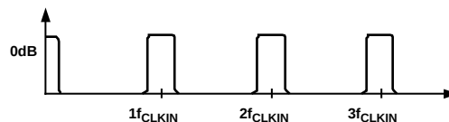
Figure 27a. Digital Filter Frequency Response
