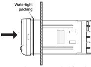
Insert the fixture into the grooves on the left and right sides of the rear case and push until it reaches the panel and is fixed in place.
