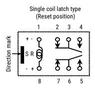
S: Coil polarity for Set R: Coil polarity for Reset
