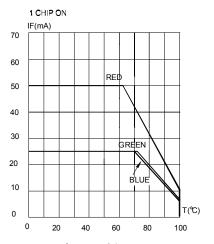
MAXIMUM FÖRWARD DC CURRENT VS, SOLDER POINT TEMPERATURE.
