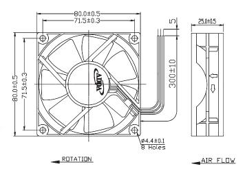
Frame:Plastic(UL:94V-0) Impeller:Plastic(UL:94V-0) Lead wire:UL1007AWG24
