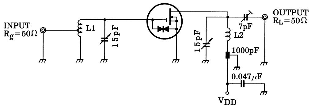
L1: 1.0 mm $\phi$  silver plated copper wire 4.0 T, 8 mm $\phi$  ID TAP at 1.0 T from coil end
