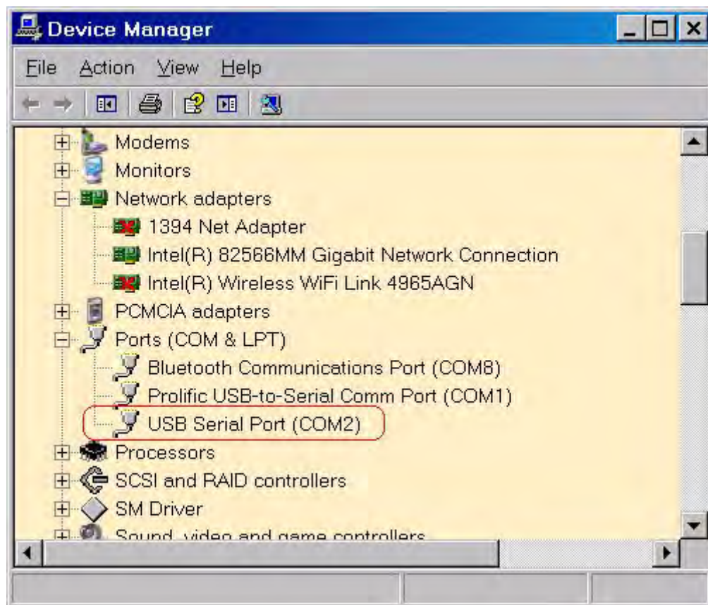
Figure 12. A Successful USB-to-UART Driver Installation
