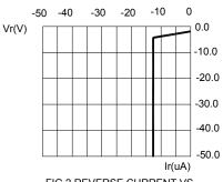
FIG.2 REVERSE CURRENT VS. REVERSE VOLTAGE.
