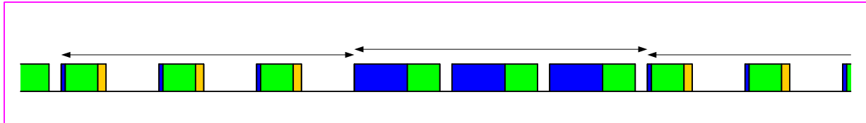
Figure 12: Extended PWM format with \text{DUAL}[5:1] = 01h (2 repetitions for each data)
