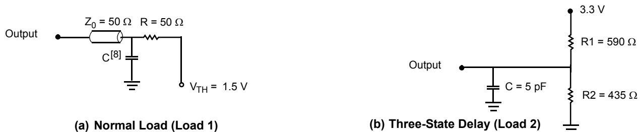
Figure 3. AC Test Load and Waveforms
