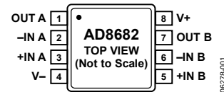
Figure 1. 8-Lead SOIC_N and 8-Lead MSOP
