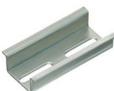
TS 35/15 mm according to EN 50022 (s = 1.5 mm)
