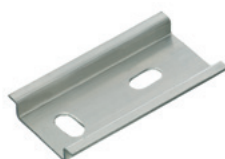
TS 35/7.5 mm according to EN 50022 (s = 1.0 mm)
