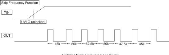
Switching frequency is changed as follows. ...  $\times 0.9 \rightarrow \times 1.1 \rightarrow \times 1.05 \rightarrow \times 1 \rightarrow \times 0.95 \rightarrow \times 0.9 \rightarrow \times 1.1$  ... It's repeated by this loop.
