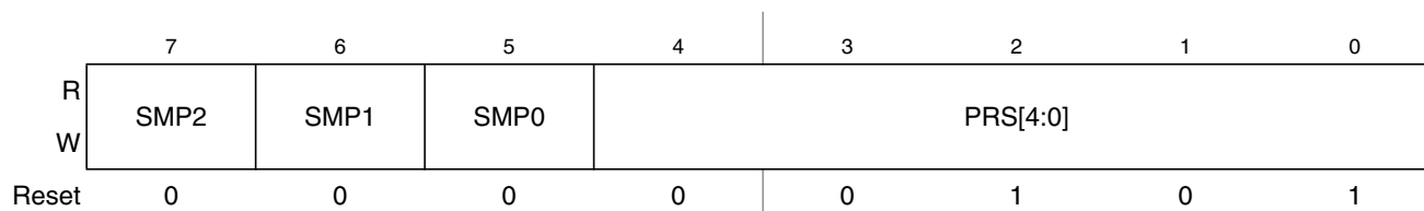
Figure 15-7. ATD Control Register 4 (ATDCTL4)
