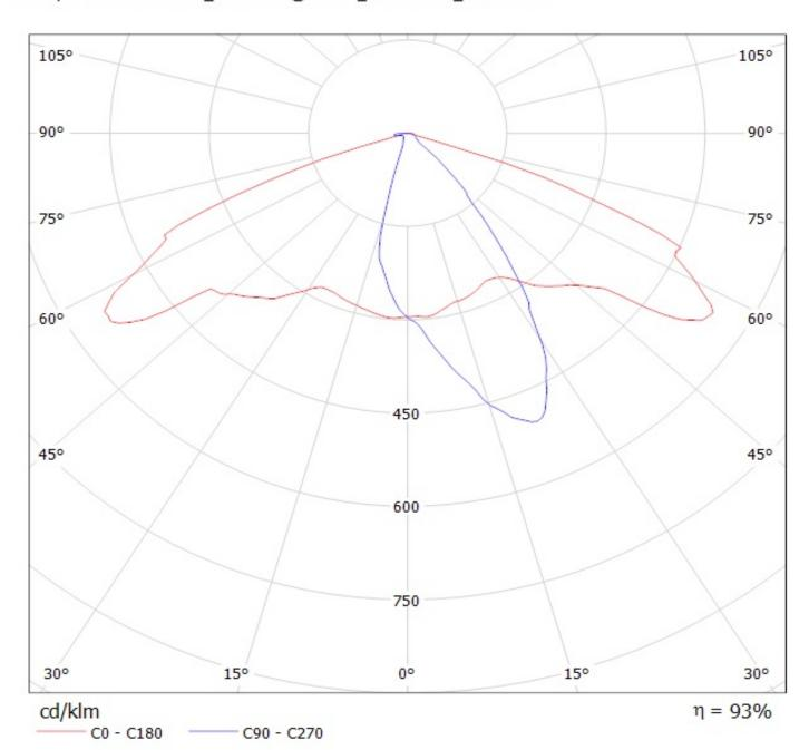
Luminaire: LEDiL Oy C13118\_&\_CA13119\_STRADA-SQ-A-T-XML (Cree XM-L 84Im@250mA) Efficiency=93% Lamps: 1 x Cree XM-L (84Im@250mA)
