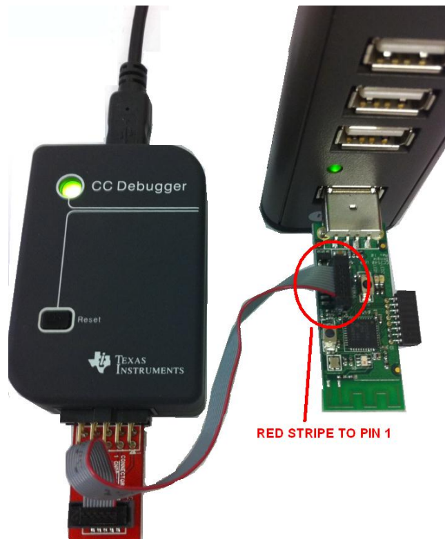
Figure 45 CC2540 USB Dongle Connected to CC Debugger
