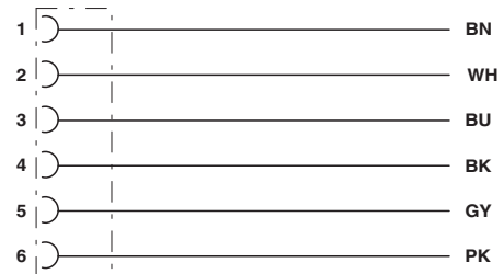
Contact assignment of M8 socket
