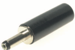
DCP3 DC Line connector. Rated 12V / 5A. With 1.3mm dia. pin
