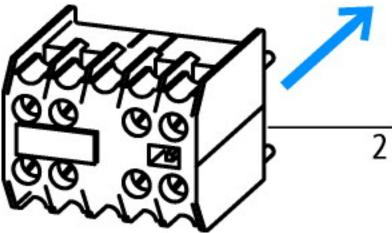
1: Suppressor 2: Auxiliary contact module
